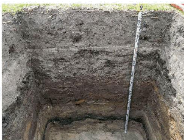
Photograph 17: TP1 end of excavation showing stratigraphy, facing north.
