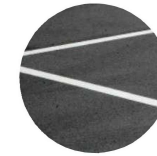
F.AS CAR PARK SURFACE 30mm ASPHALT OVER 150mm RECYCLED CONCRETE ROAD BASE TO ENGINEER'S SPEC.
