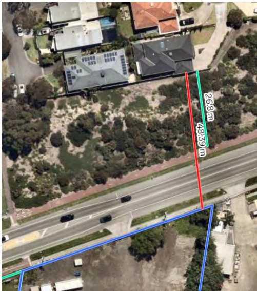
Distance between subject land and residential properties in red and minimum width of raised buffer in green (source – Nearmaps)
