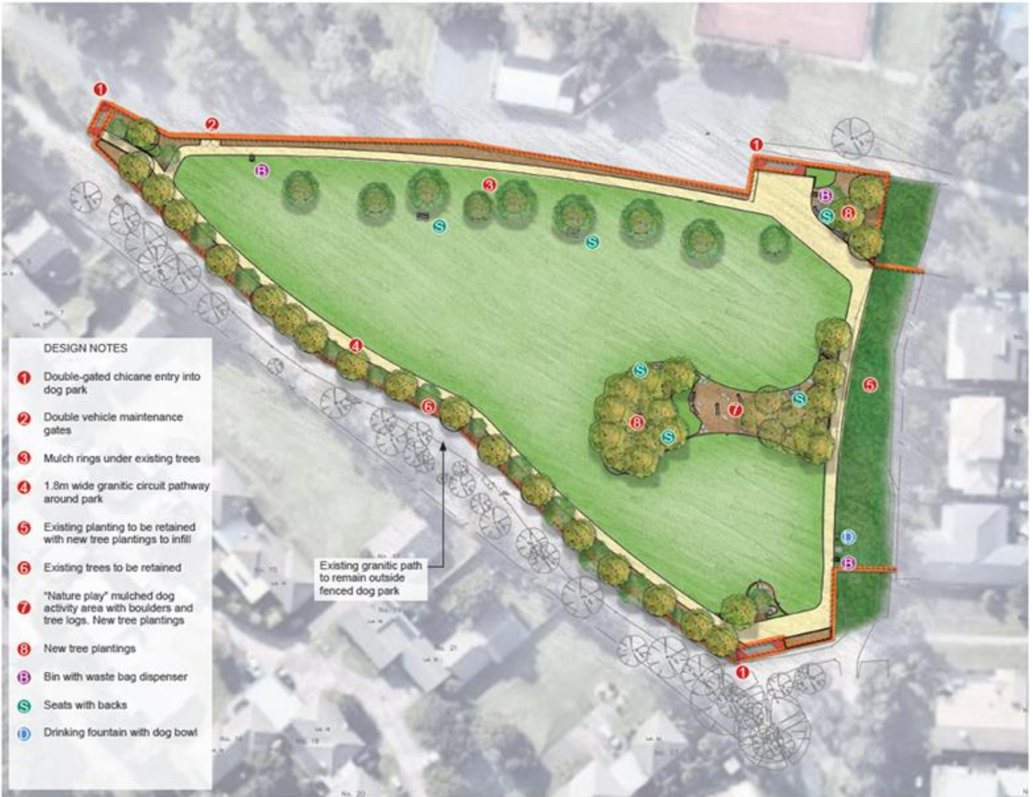
New Fenced Off-Leash Dog Park at Roy Dore Reserve, Carrum - Landscape Plan
